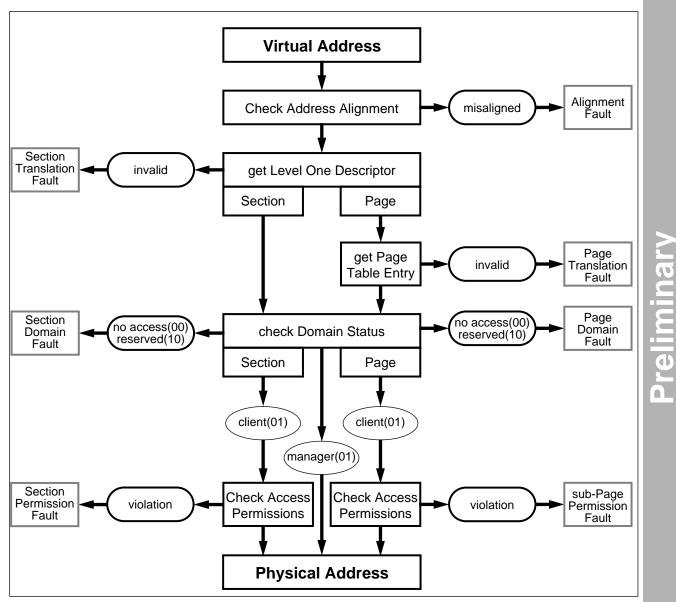
Figure 7-10: Sequence for checking faults
